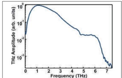
**Tera-SED3** emission spectrum at 10 V DC bias and 0.7 nJ pulse energy, acquired with Laser Quantum GmbH (formerly Gigaoptics) ' High-Speed ASOPS technique.
